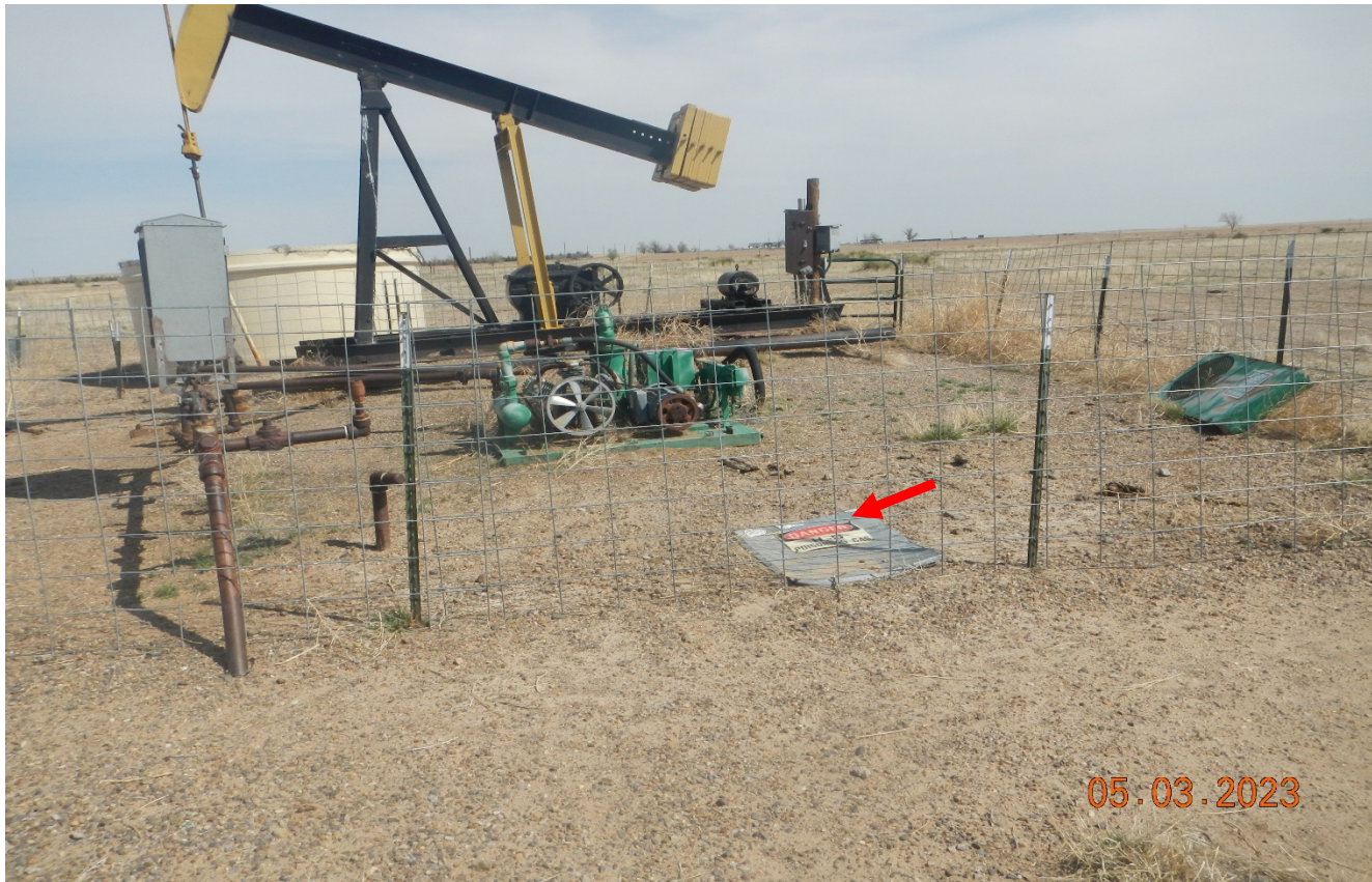
Photo 3. Facing toward the pumpjack. The H2S sign is laying on the ground.
