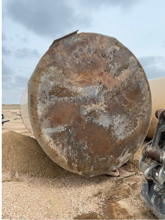
5 – QC A 32-19 base of west AST; some rust, no penetration
