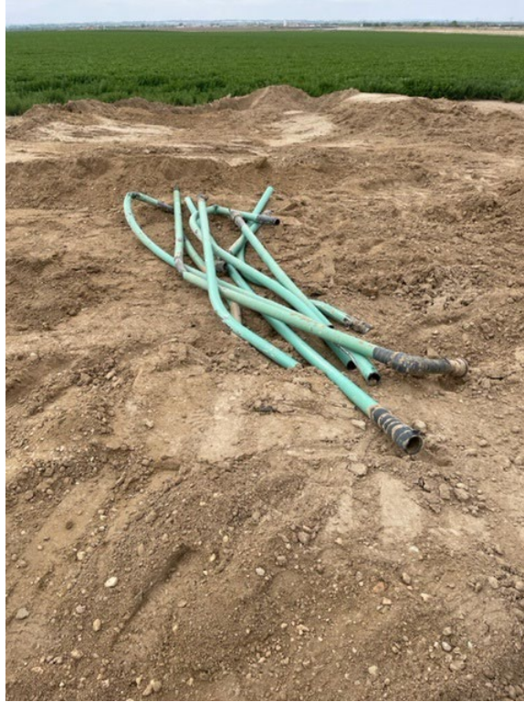
11 – QC A 32-19 dumlins with green epoxy coating in good condition
