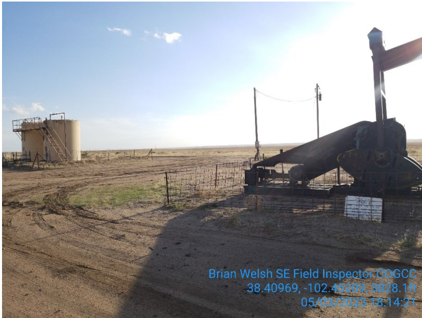
1. Pumping unit and tank battery
