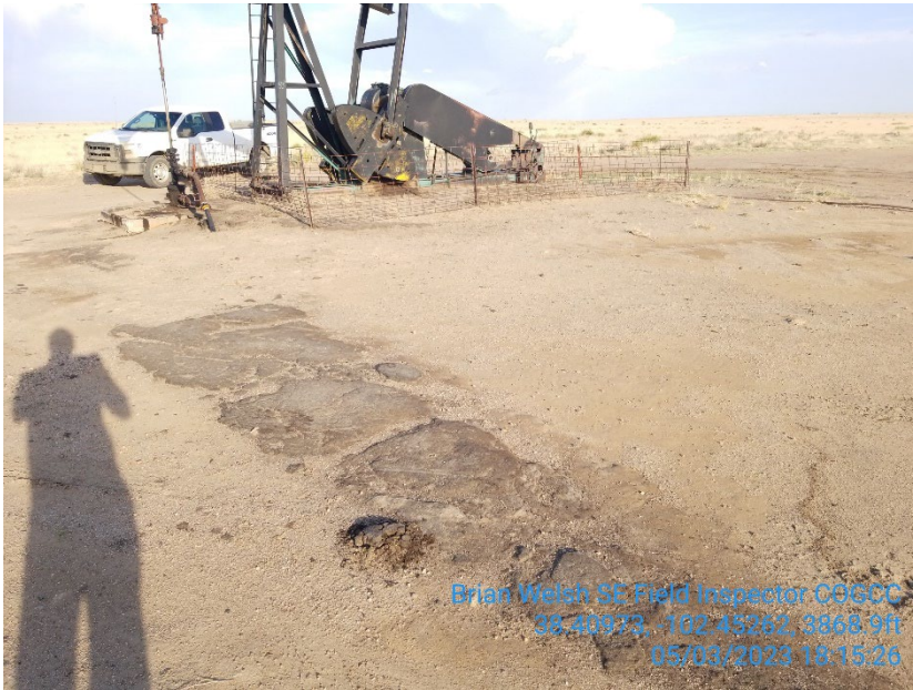
3. Stained soil on west side of wellhead
