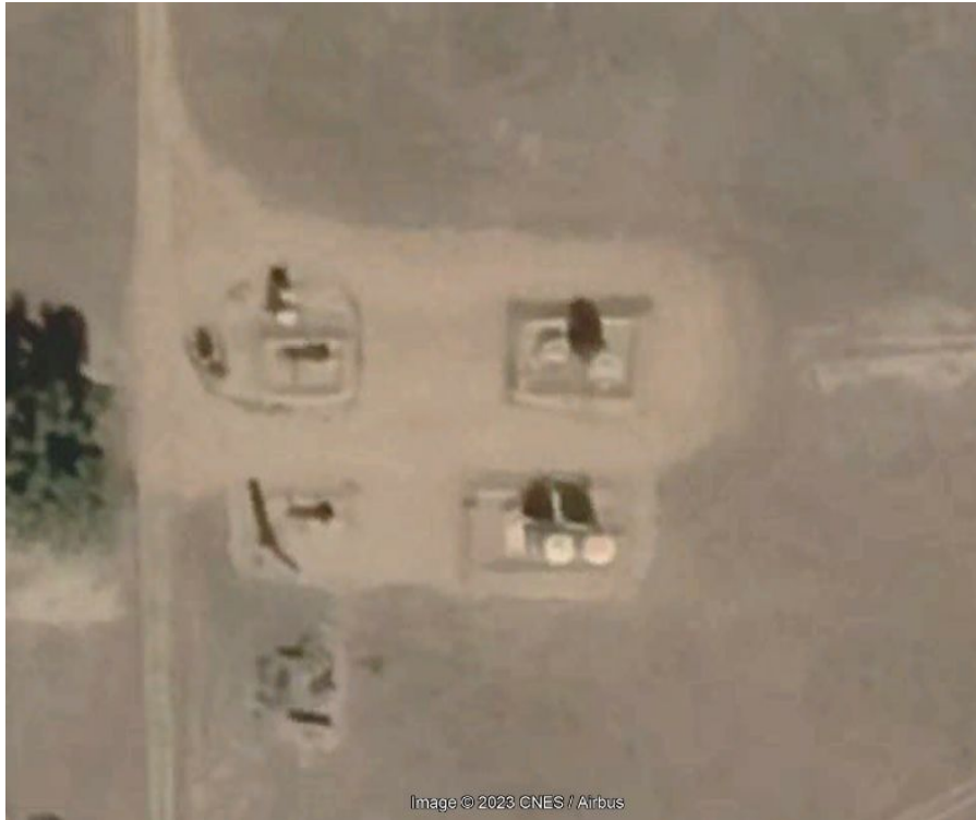
Photo 5. Google Earth aerial imagery from 9/25/2018 illustrates the shared tank battery. PDC's portion of the tank battery is the northern half, while Noble's portion is the southern half.
