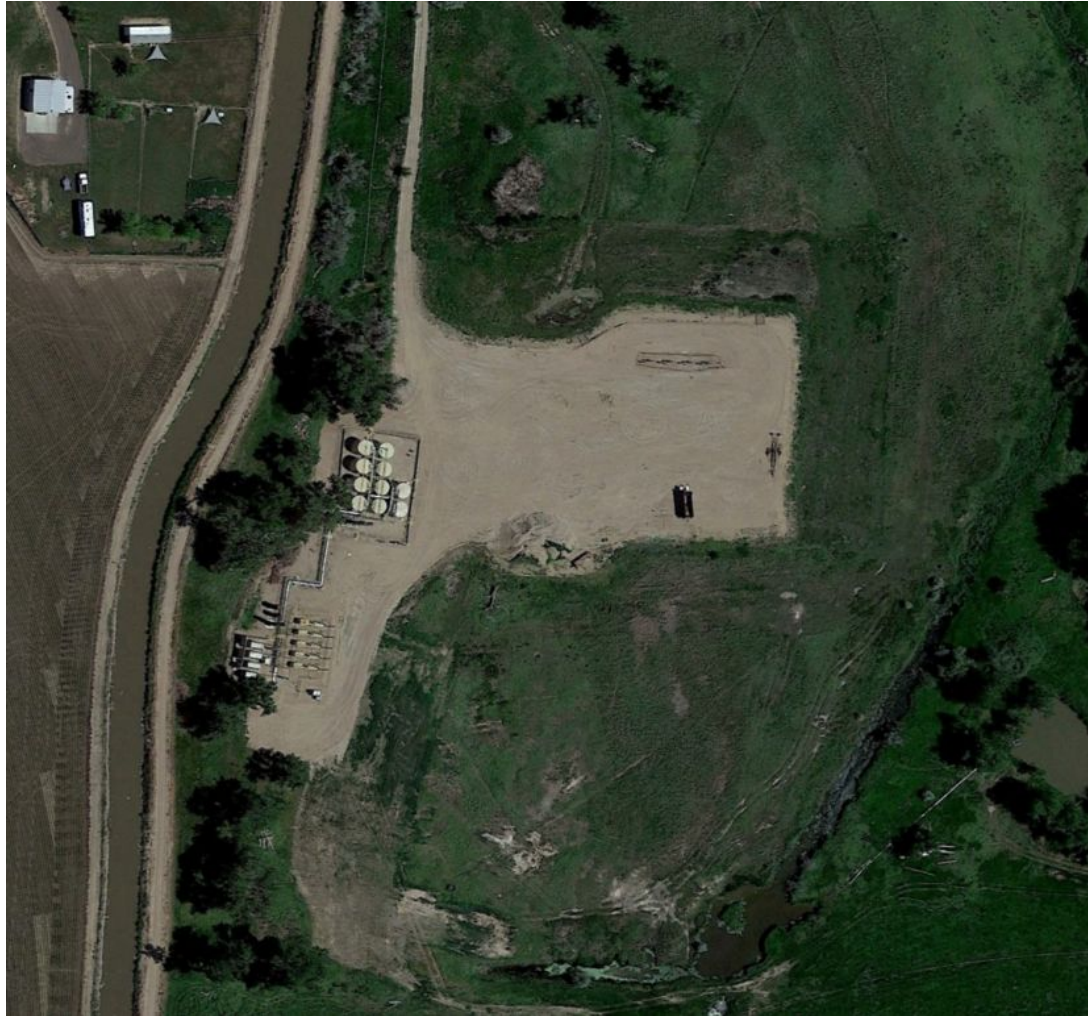
Photo 3. Google Earth aerial imagery from 6/11/2021 illustrates the Operator has plugged the original well (123-35776) but has failed to further reduce all areas not needed for production operations. Operator should have performed interim reclamation by no later than 10/10/2020. The southern/southeastern well pad can be further reclaimed per Rule 1003.
