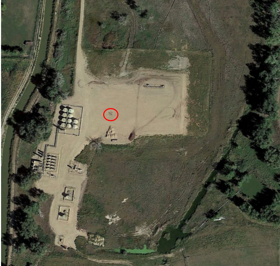
Photo 2. Google Earth aerial imagery from 9/12/2018 illustrates the Operator performed interim reclamation activities to reduce all area not needed for production operations.
