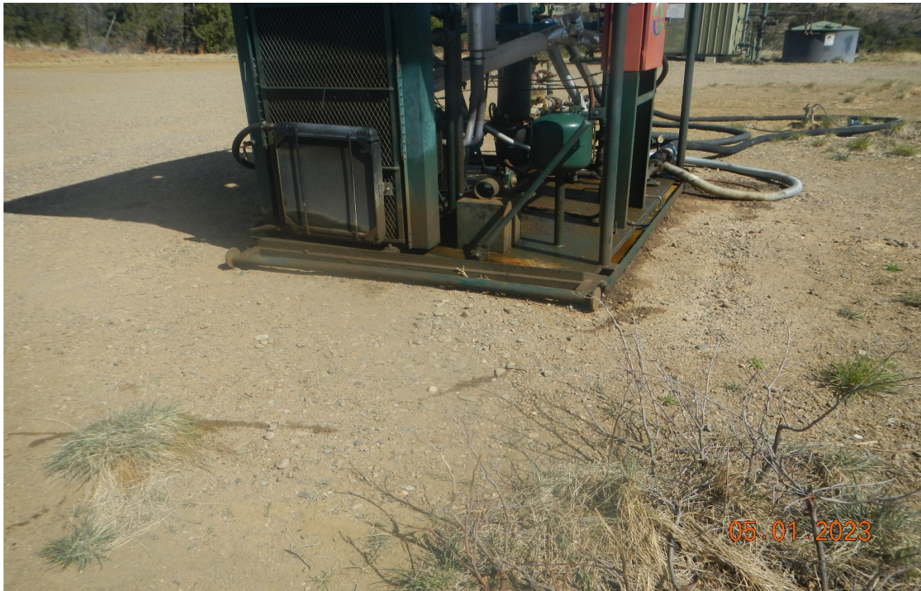
Photo 5. There is oily fluid in the engine skid that needs to be cleaned up.
