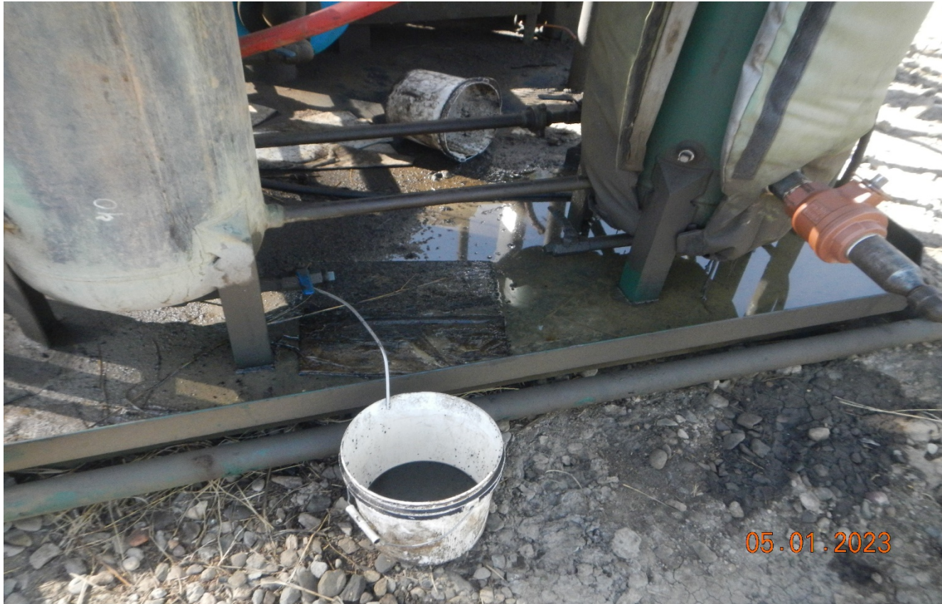
Photo 2. There is a bucket with oil not in containment and should be covered for wildlife protection.
