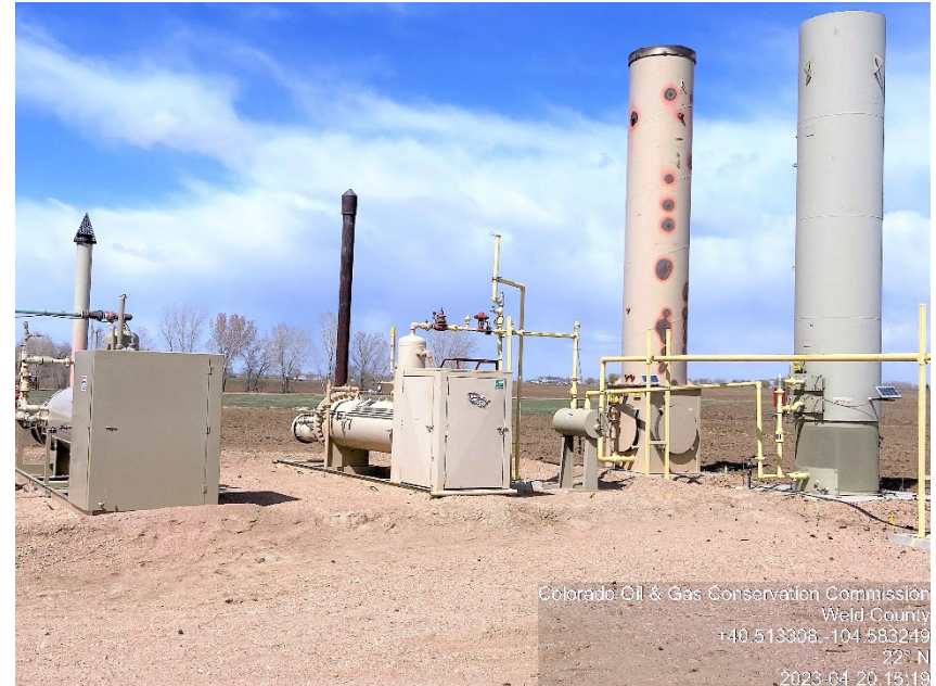
Photo #4 Dyer USX A 05-14 Battery site Active Separator(s), ECD(s) prior photo
