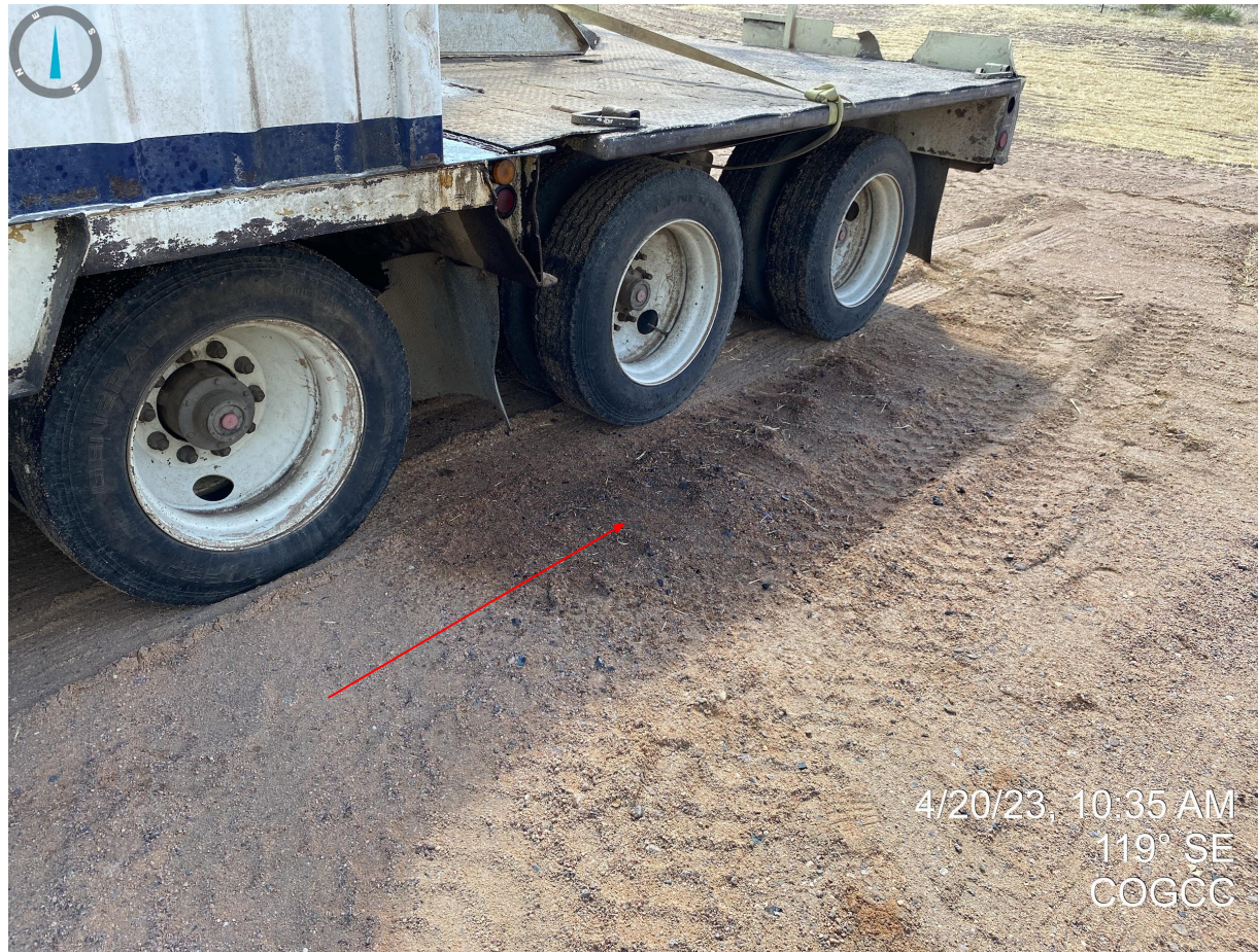
Photo 19. Stained soil from leaking equipment that will need to be properly disposed of per Rule 905.e.
