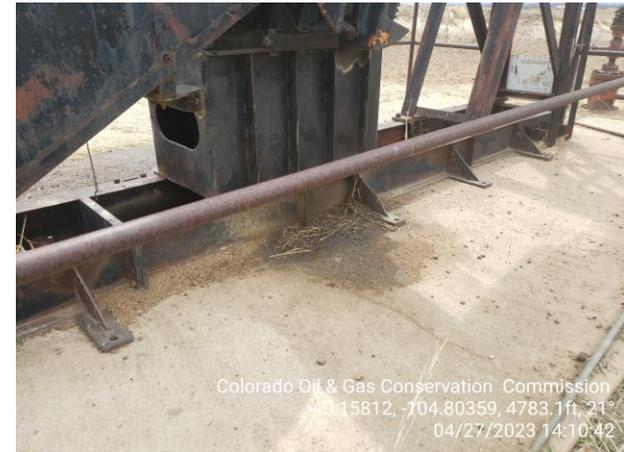
**Photo 5 Oil staining on Concrete pad from leaking PJ gear box .**
