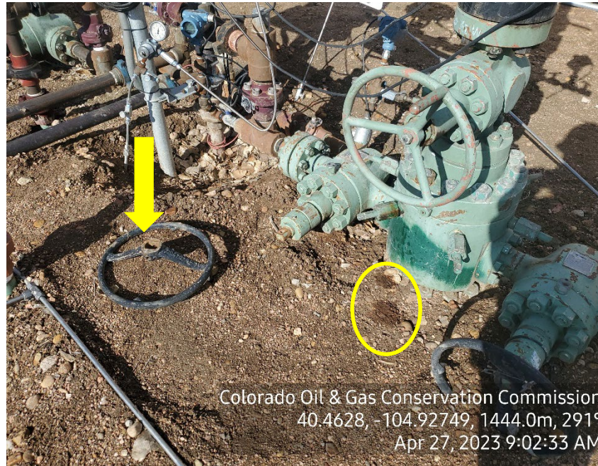
Photo 3: Stained soil, unused/disconnected equipment
