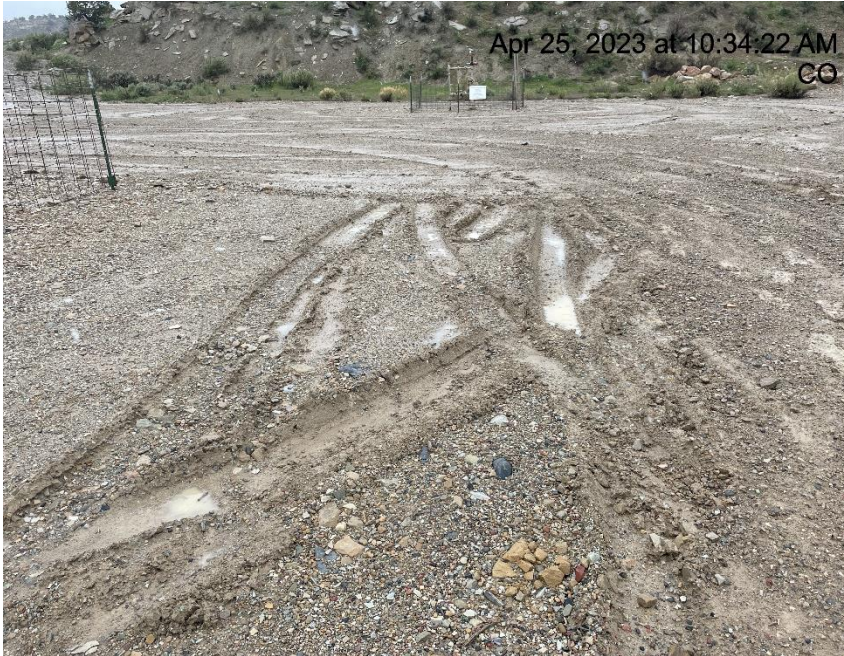
Photo # 6318 Lack of stabilization/compaction
