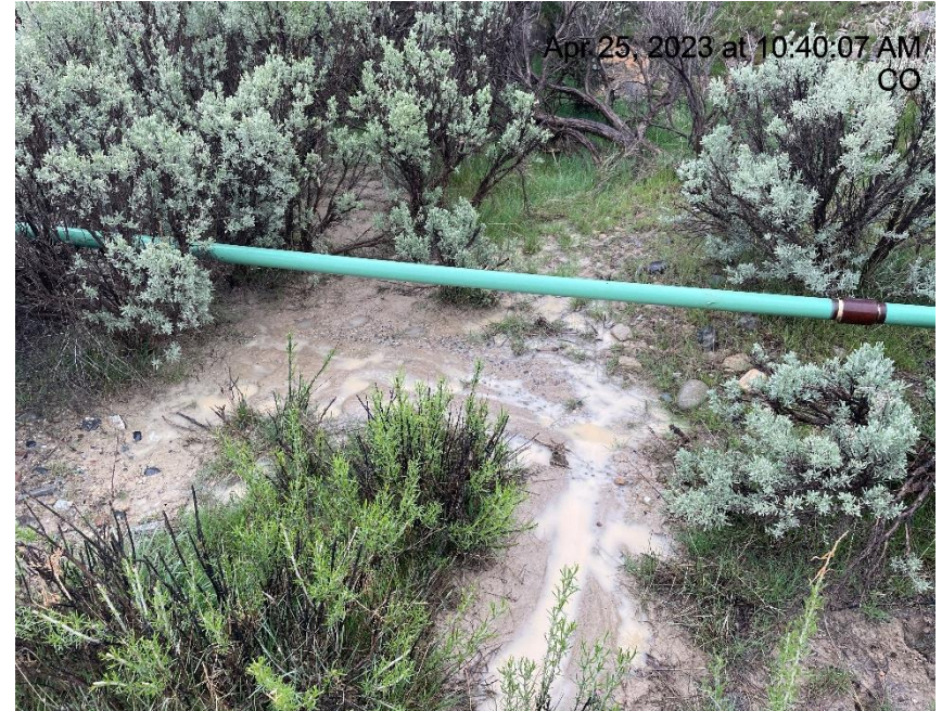
Photo # 6336 Erosion & transport of sediment off location
