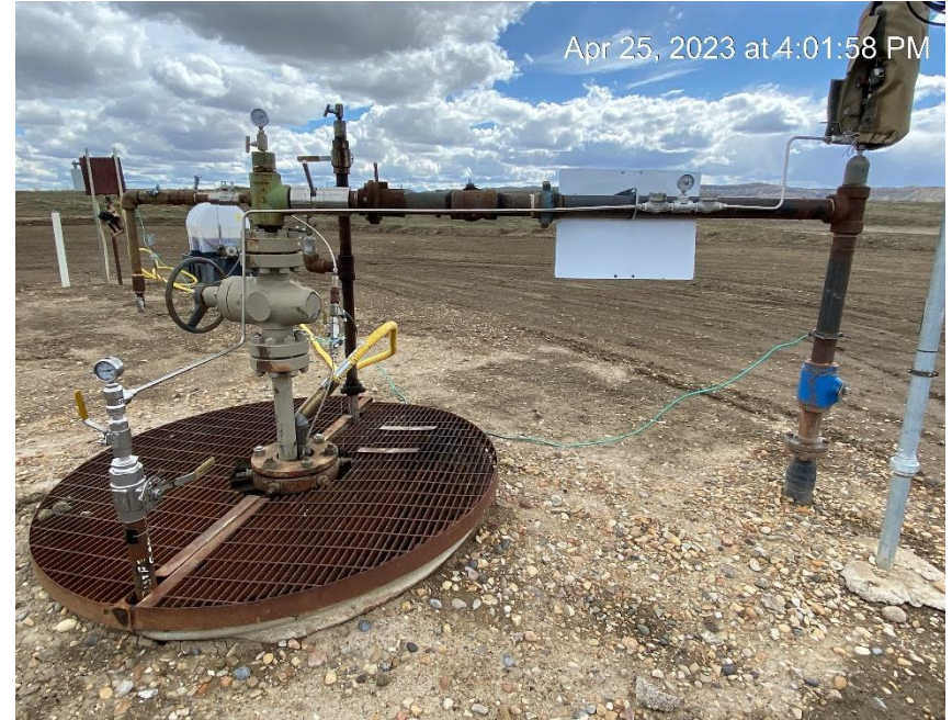
Surface casing hooked into flowline
