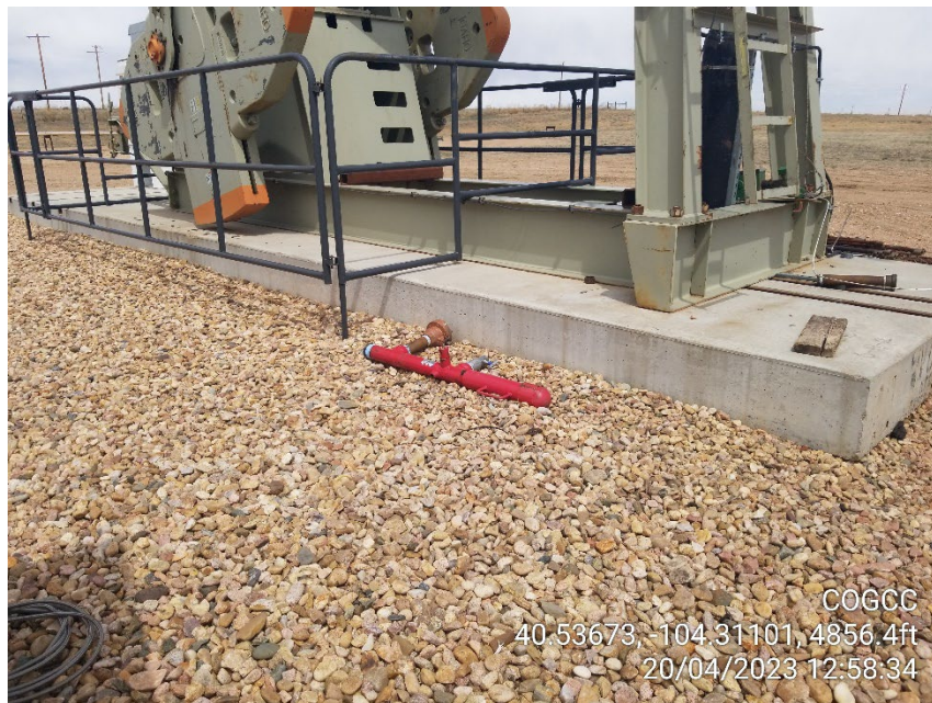
Photo 9 – Plunger Lubricator Cap
