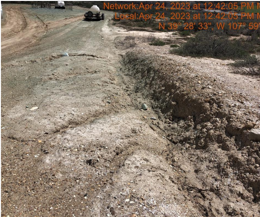
Photo #9719 Rill erosion occurring on location.
