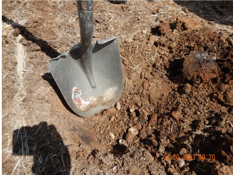
Photo 7. Photo taken from a portion of the access road. COGCC staff dug ~5-6" down and hit a refusal area of gravel. It does not appear the Operator removed all the gravel from the access road. This was not observed in reference areas. Refer to Photo 8.
