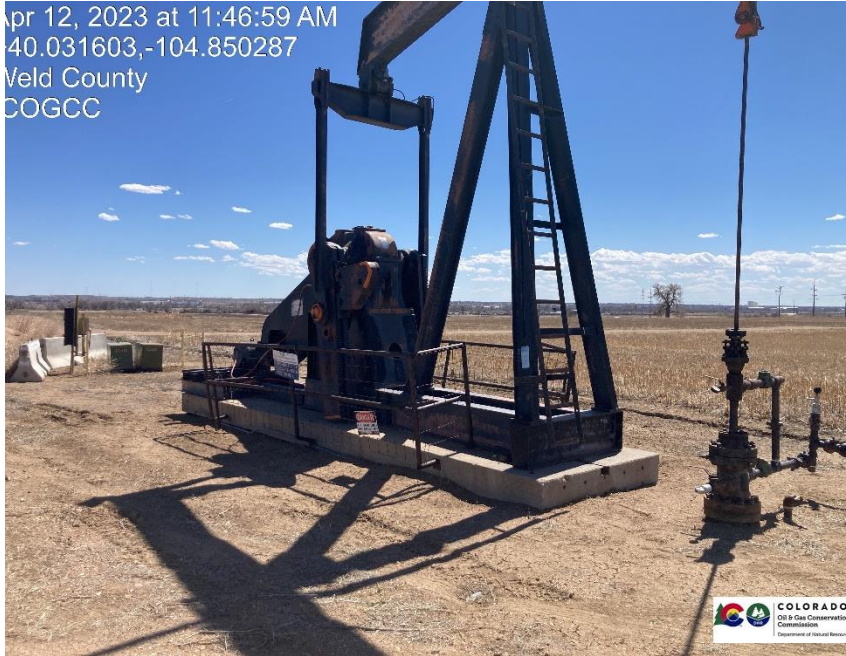
Pic 1 wellhead / pump jack
