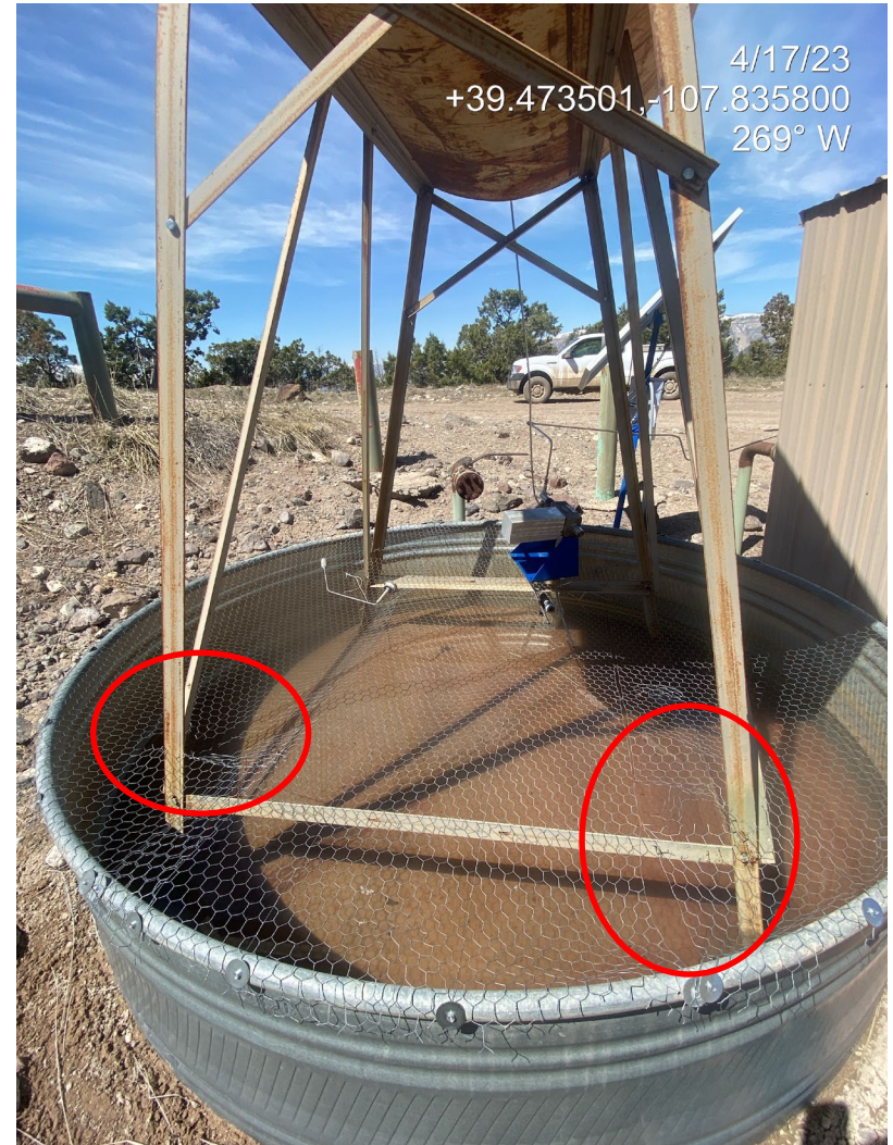
Photo 4. Photos show a bull plug not installed on a tank drain (left) and wildlife protection BMPs in disrepair (right).
