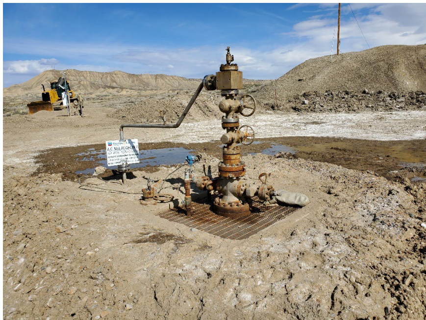
Injection wellhead
