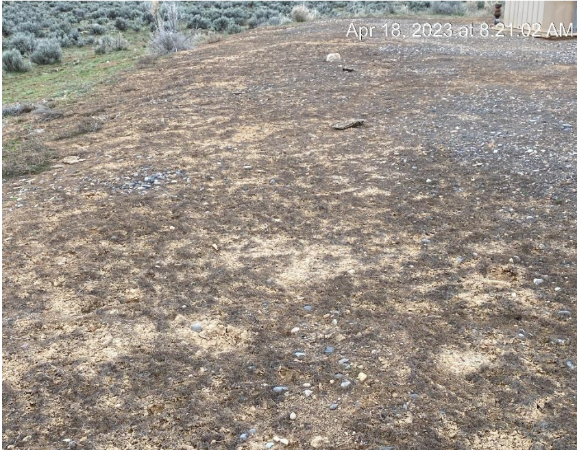
Lack of Stormwater BMPs to control sediment migration
