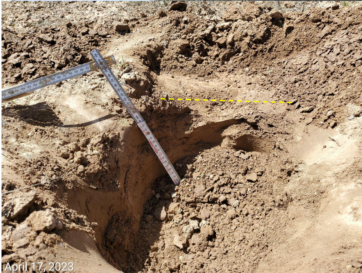
Photo 6: Continued from photo 4. Photo shows Location has not been decompacted; zone of compaction, represented by the dotted yellow line, observed ~ 3 inches below ground surface.
