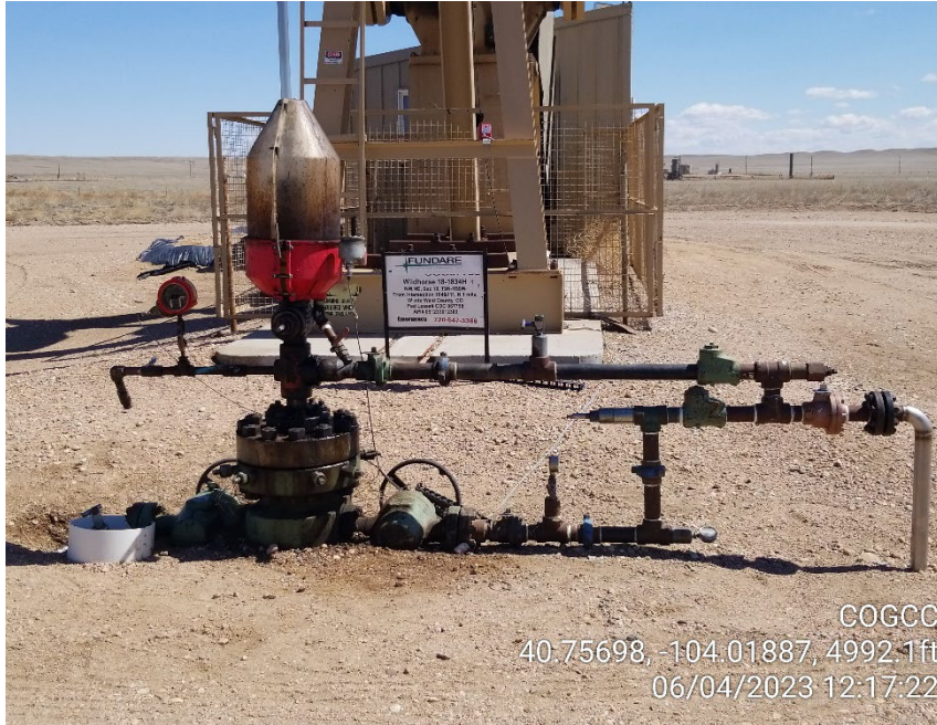
Photo 1 – Wellhead – Stained Soil
