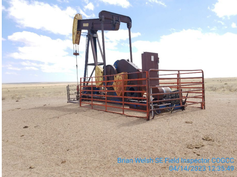
1. Pumping unit with panels installed
