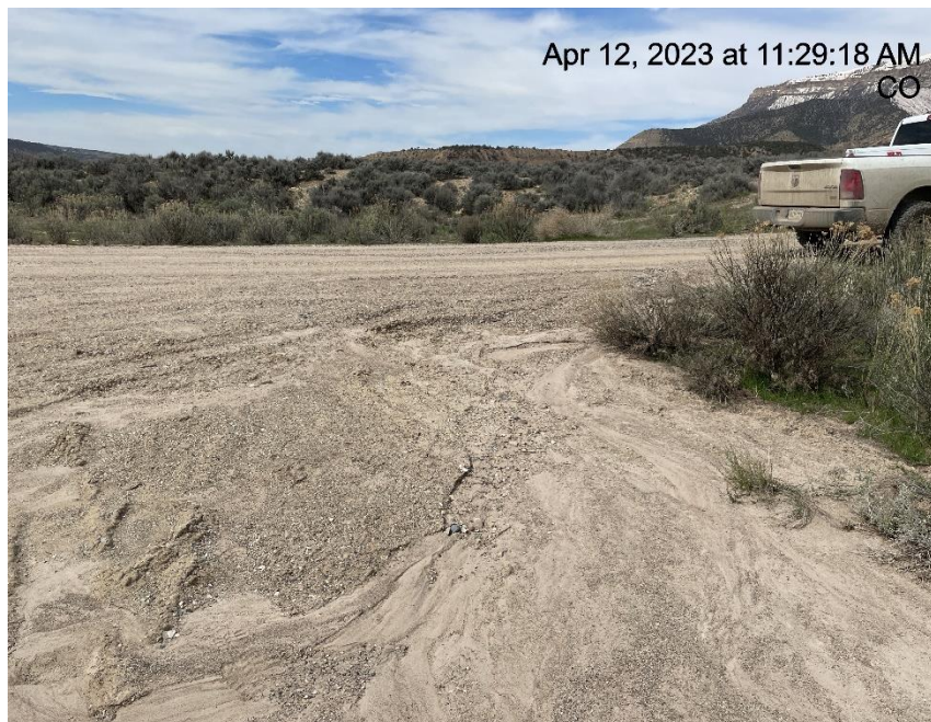
Photo # 5079 Erosion & transport of sediment onto location
