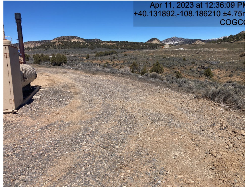
Location lacks BMP's to prevent sediment migration
