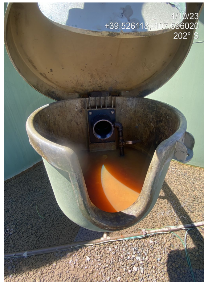
Photo 3. Photos show production areas (left) and a load line without a bull plug installed (right).
