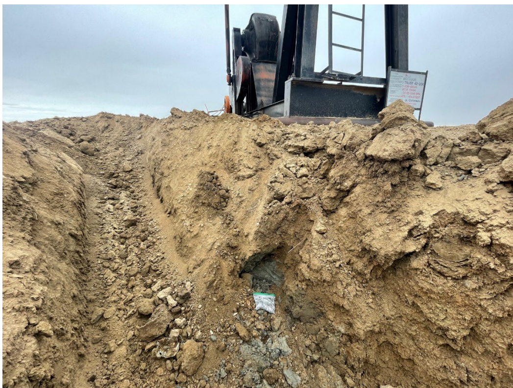
FL2) Sample location FLN1-3.5, soil staining and odor present- facing northeast
