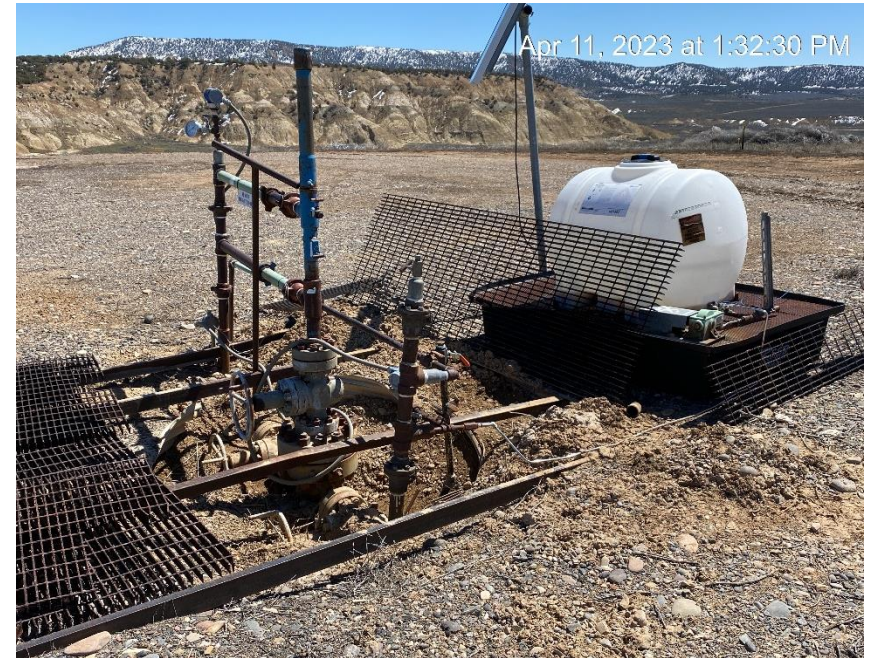
Open cellar around wellhead
