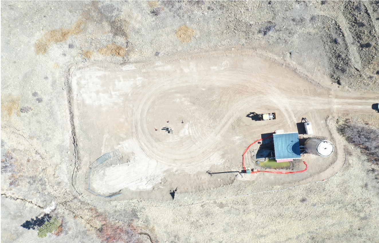
Photo 1. Drone aerial photo of the location showing the excavated areas of the remediation project.
