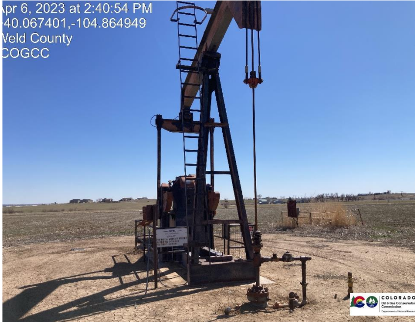
Pic 1 wellhead / pump jack
