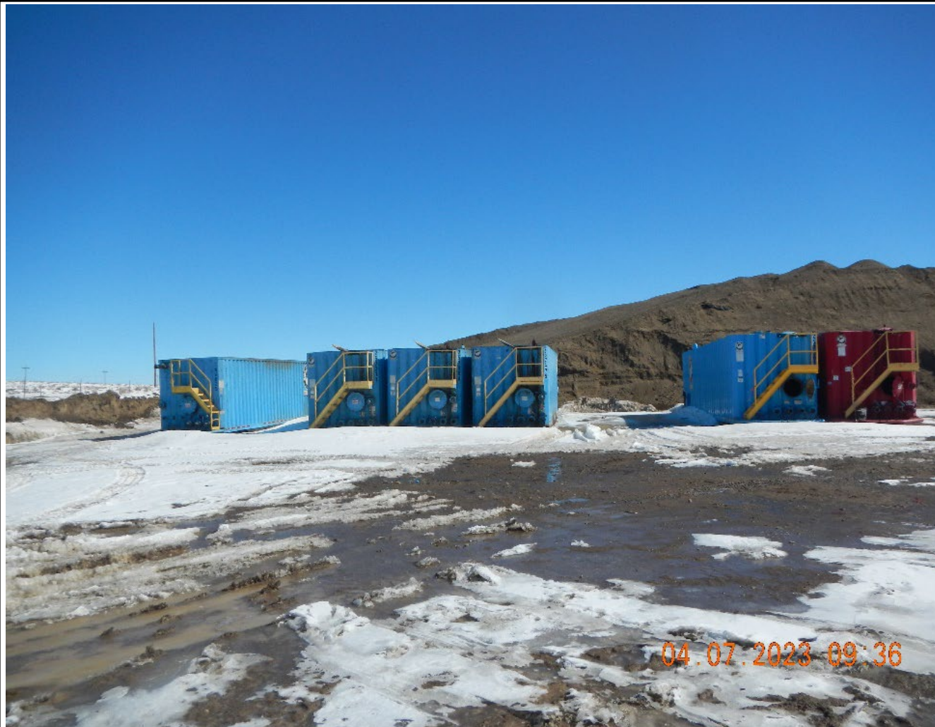
Photo #9 Frac tanks on North side of location. Appeared not plumbed. Note: cleanout hatch open on some tanks.
