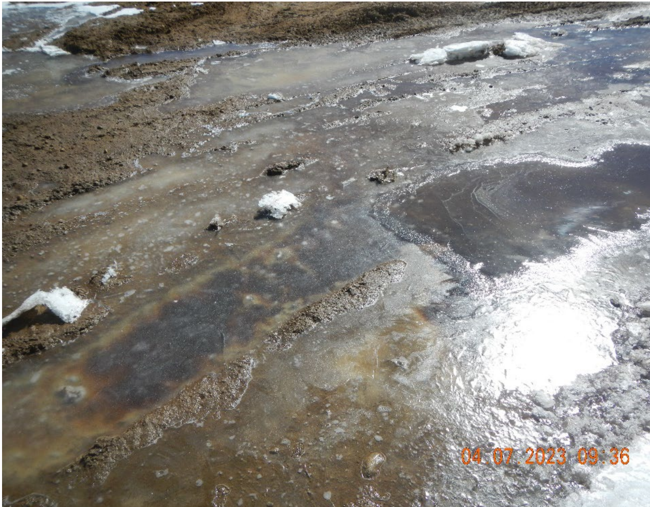
Photo #12 oil on ground near caged wellheads. Oil was on water below ice. Corrective Action; This area shall be documented on a Remediation workplan (Form 27).
