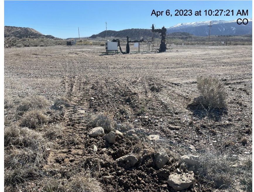
Photo # 4474 Failure to minimize surface disturbance/vehicle tracks into interim area/transport of sediment.
