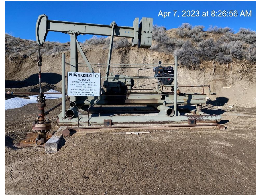
Wellhead and pumping unit
