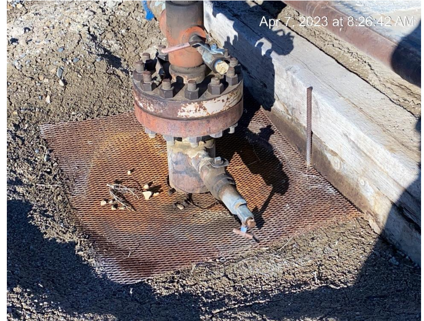
No Bradenhead. Surface casing only.
