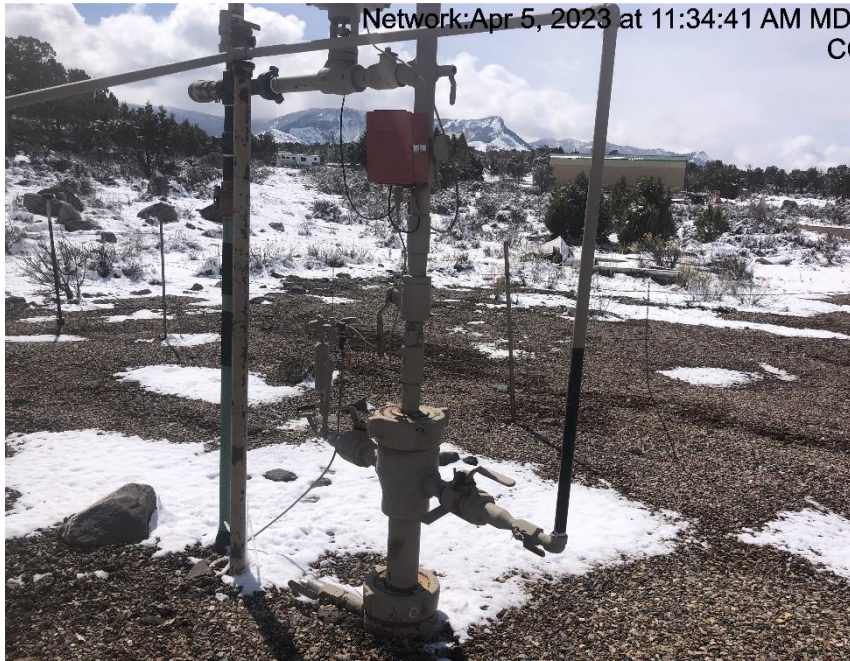
Photo #9534 Domestic tap is derived from the back side casing valve.
