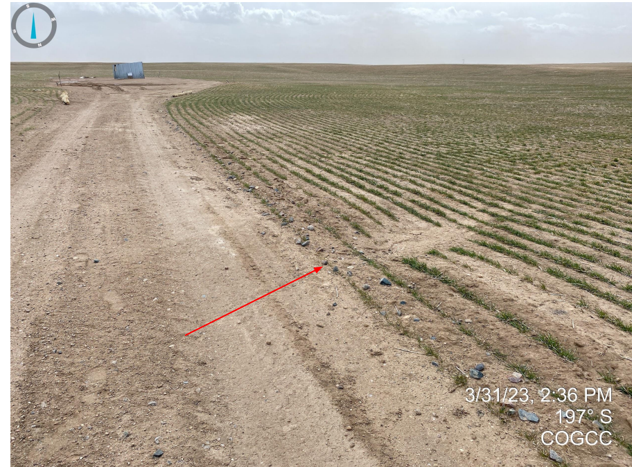
Photos 4 & 5. Rill erosion evident (red arrows) with no stormwater BMPs identified.
