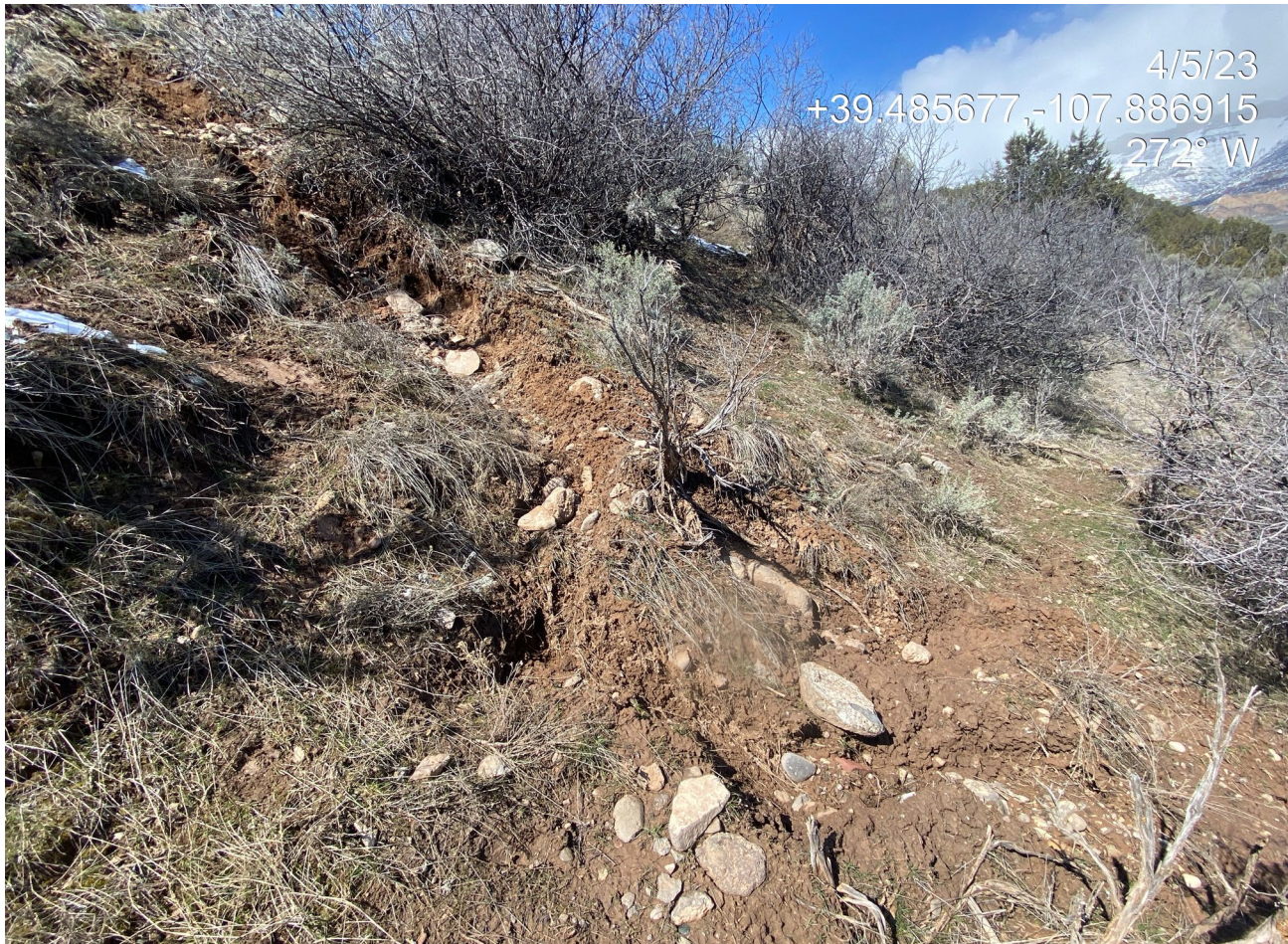
Photo 11. Photo taken just downslope of Photos 9 and 10 shows concentrated flows from the drain pipe resulting in rill erosion, sediment transport and offsite degradation.
