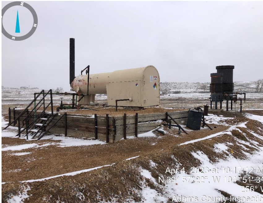
Photo# 5 Separator & ECDs.
