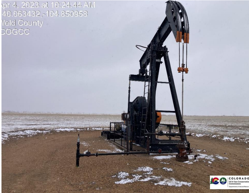
Pic 1 wellhead, pump jack.
