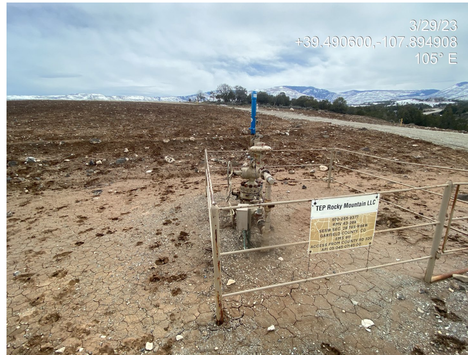
Photo 2. Photos show production areas. Note the sediment that has been transported from the southern interim area around the wellhead (right).
