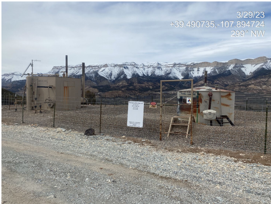
Photo 2. Photos show production areas. Note the sediment that has been transported from the southern interim area around the wellhead (right).
