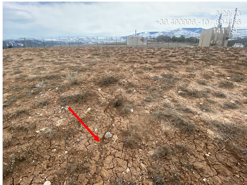
Photo 11. Photo shows pedestaling and a rill in the northern interim area indicating erosion.
