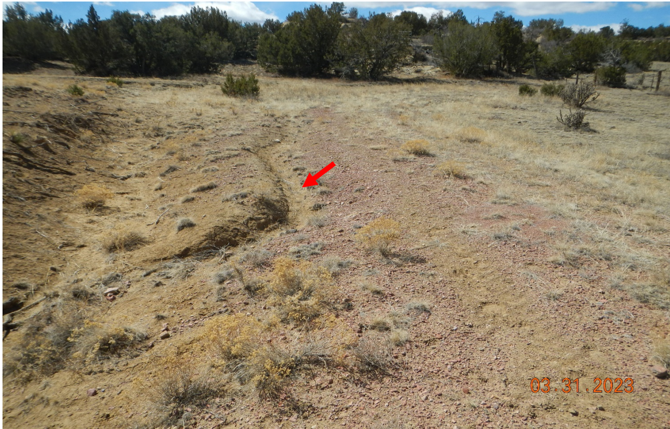
Photo 3. Facing southwest along the access road. This portion of the access road has not been reclaimed and there is erosion shown at red arrow.
