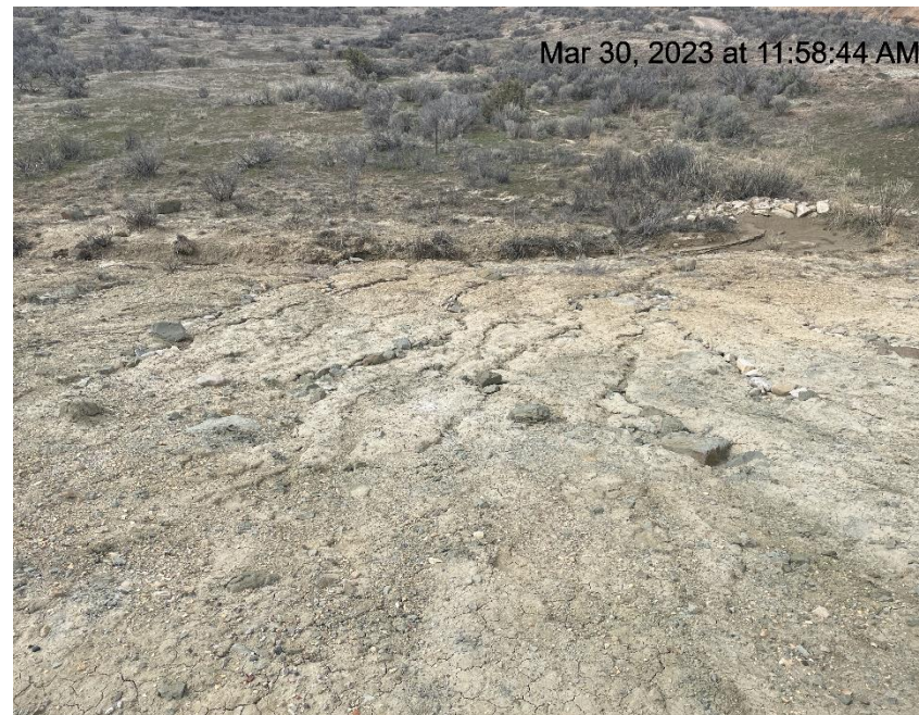
Photo # 3742 Rill erosion & transport of sediment (NW area of location)
