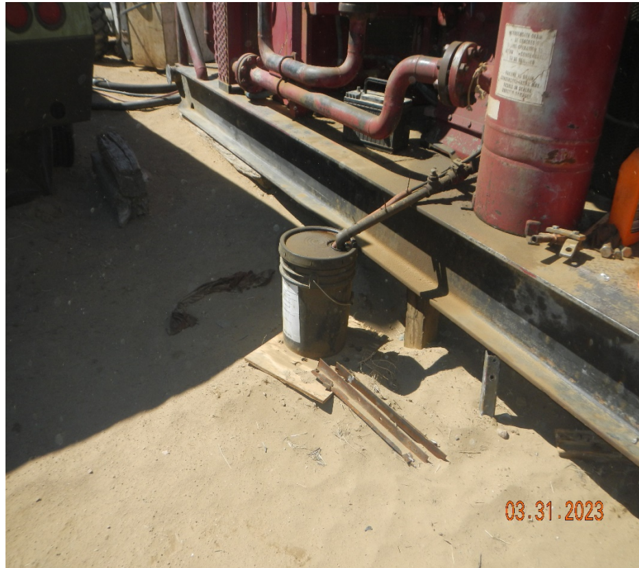
Photo 10. There is oil leaking out of the equipment being captured by buckets which could easily tip over and spill.
