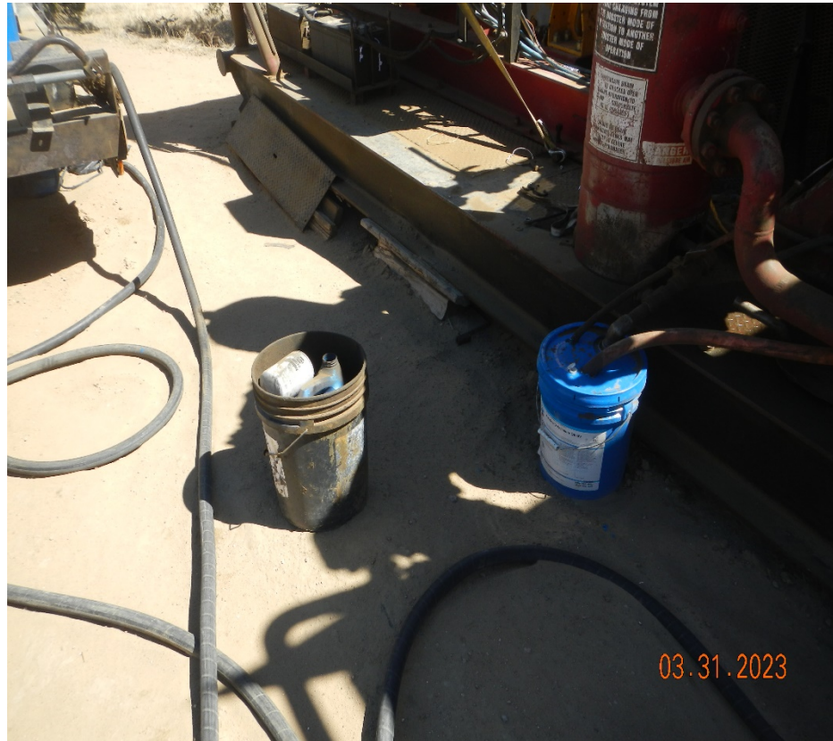
Photo 14. There is oil leaking out of the equipment being captured by buckets which could easily tip over and spill.
