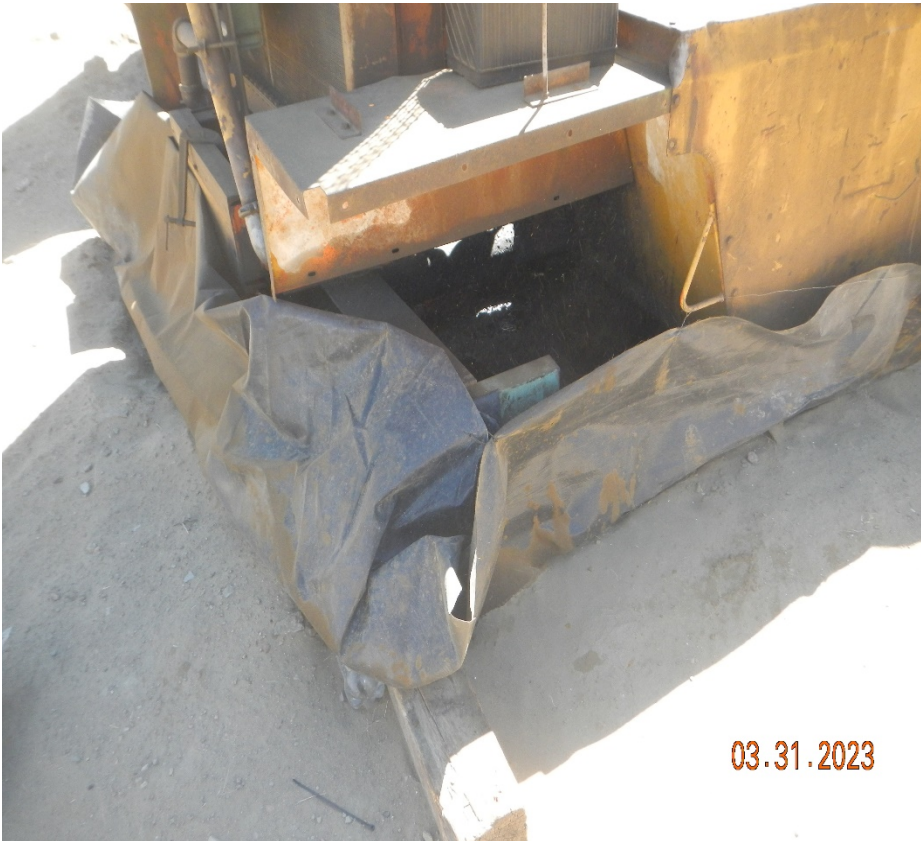
Photo 5. The equipment which is leaking fluids has liner that has been wired up but this is not adequate for containment and fluids in the liner need to be cleaned up.
