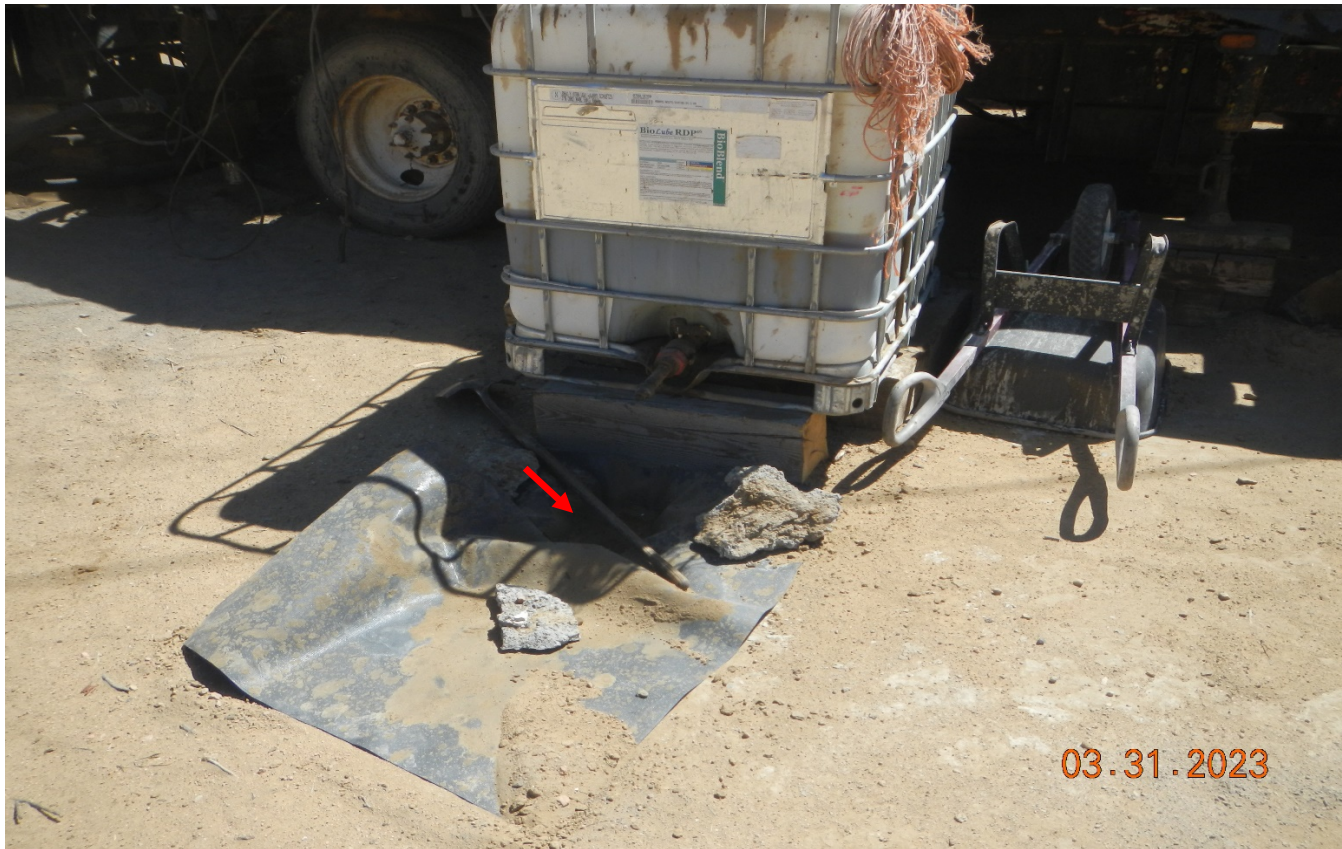
Photo 26. There is no containment for this chemical tote. A plastic liner was placed out the outlet which will not control a potential spill. Additionally there is a puddle of oily fluid at the outlet shown at red arrow.
