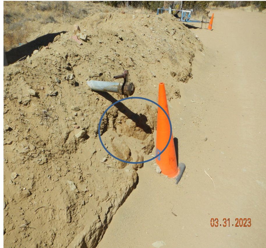
Photo 17. There is still oil stained soils at the tank pipe outlet shown at circled area of darkened soil..
