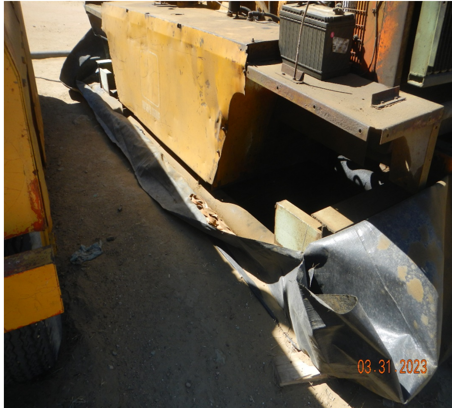
Photo 6. The liner on the other side of the equipment is laying on the ground and stormwater could easily wash out oily fluids onto the ground..
