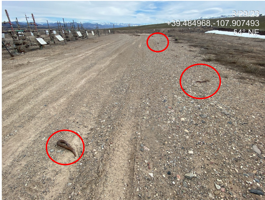
Photo 4. Photos show unmarked anchors to the south of the wells.
