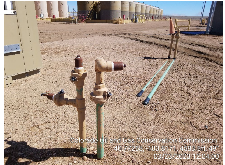
Photo 18 – Unmarked Riser at Air Unit
