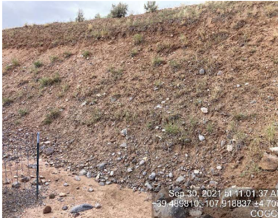
Photo 7. Photos taken to the west of the battery show the cut slope on 9/30/2021 (left) and on 3/29/23 (right). Erosion has progressed to form a large rill on the slope. Note three sagebrush at top of slope for reference.
