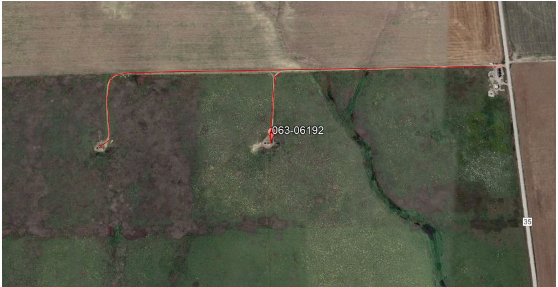
Photo 15. Google Earth aerial imagery illustrating the access roads (red) that remain and will need to be reclaimed per Rule 1004. Previous inspection (Doc #696200704) provided photos showing that the lease/access road did not exist pre-oil and gas development.
