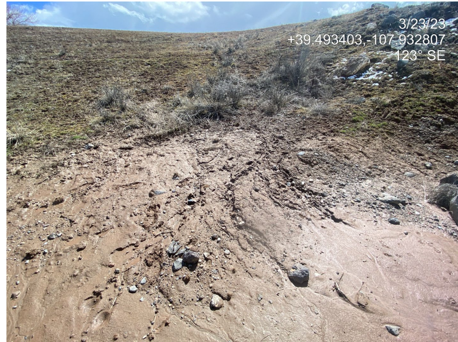
Photo 7. Photo shows sediment runoff from the working pad area into interim areas (left) and from cut slopes/interim areas where rill erosion is occurring onto the pad (right).
