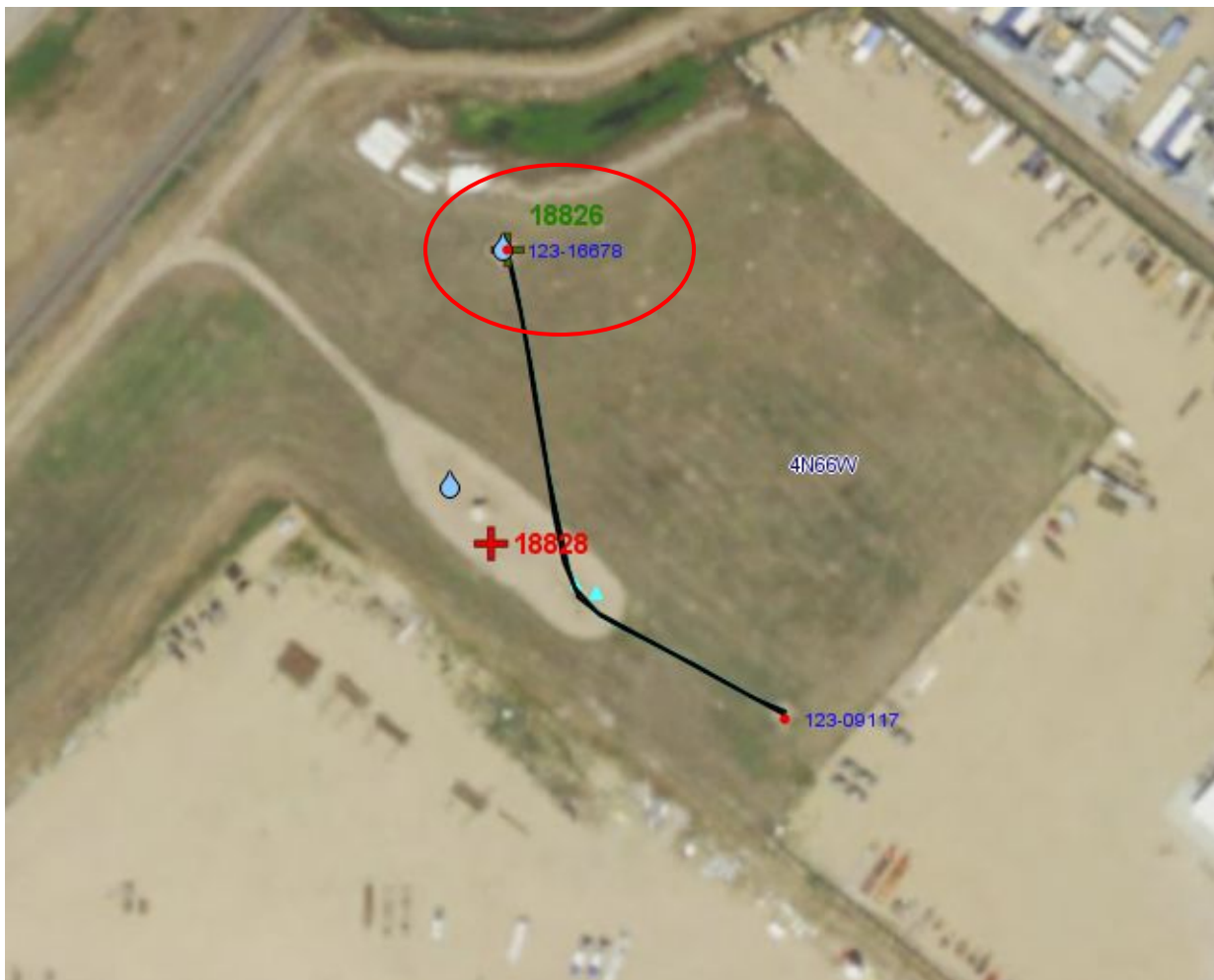
Photo 5. Photo illustrates the well location (red circle) and off-location flowline to the the tank battery.
