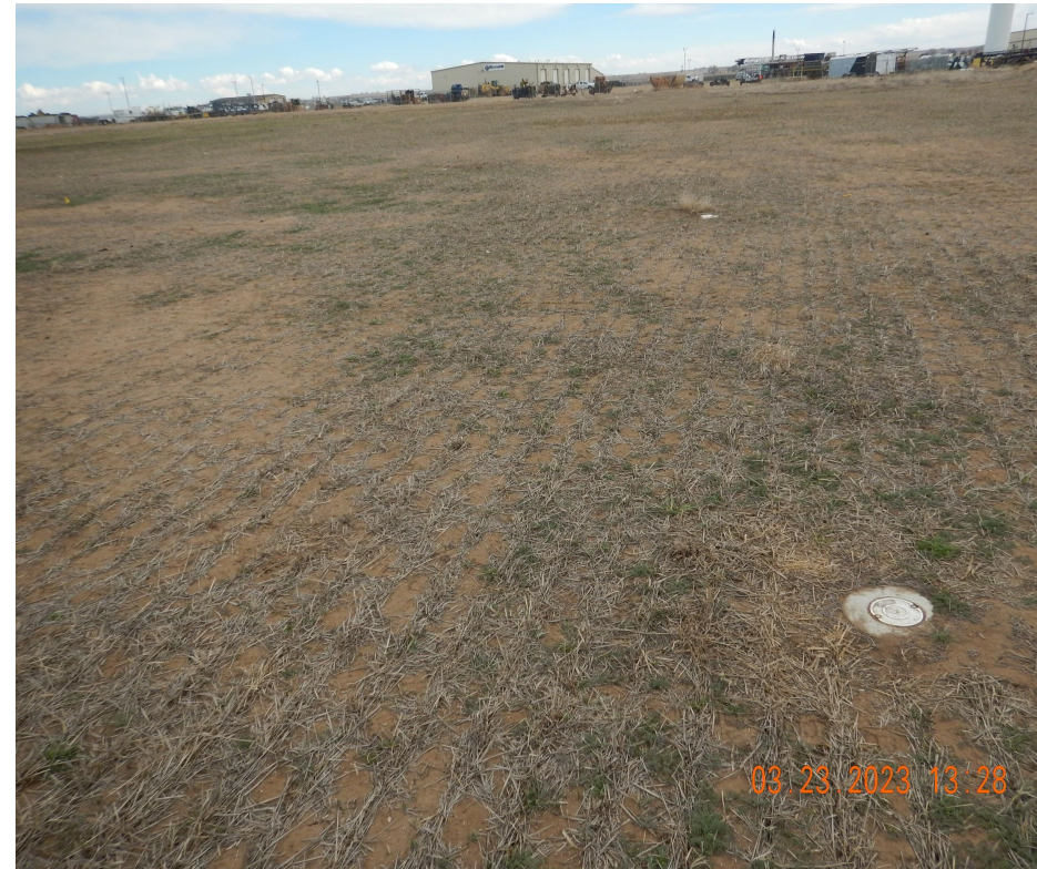
Photo 4. Photo taken from the tank battery, facing Southeast. Photo illustrates 1 of the 12 groundwater monitoring wells that have been installed.
