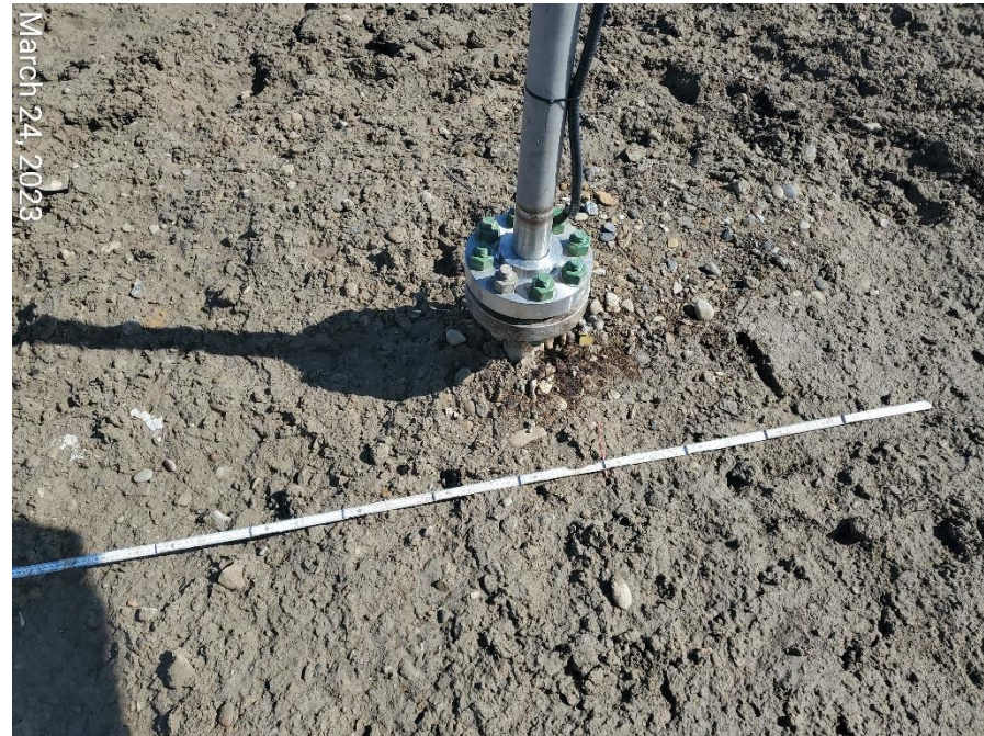
Photo 11: Photos shows stained soils around production equipment.
