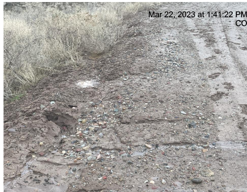
Photo # 2888 Rill & tunnel erosion (upper tier of pad, south side)
